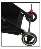
To set your parking brake, push down on the brake pedal.
