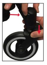
To remove the rear wheels you will need a phillips screwdriver. Unscrew the locking screw on the underside of the frame and pull the wheel out.
