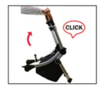
Lift the frame up until it locks in place. Listen for the frame to click into place.
