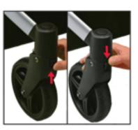
To set your front wheels to not swivel (locked position), slide the swivel lock up. To unlock, slide the tab down.
