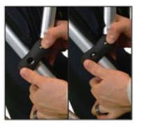
Then line up one of the canopy ratchets over the post on the seat frame, (lining up the hole), and angle it onto the frame. Repeat on the other side.
